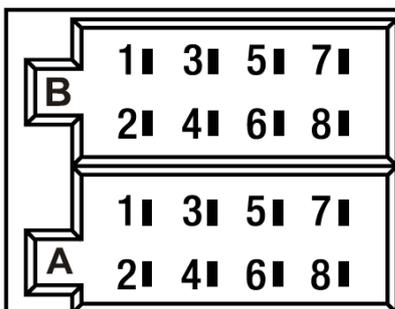
**Note:** The black wiring remote cable/socket (A) on the unit is for the commander MRC21 and it is also compatible with the MRF90 receiver.
