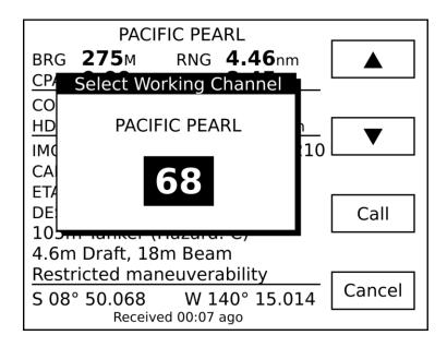
Use the arrow buttons to scroll up/down to the desired channel. The last used working channel is remembered and becomes the default for subsequent calls.
