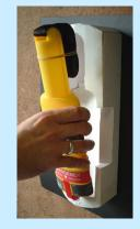
Pull down firmly on the red activation clip to turn the SART 'ON'. The LED will flash slowly. When in range of a radar signal, the LED will flash rapidly.
