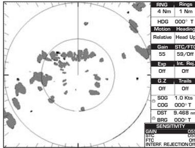
Fig. 1.7.4.4g - Transmission Trigger Delay tuning (VIII)
