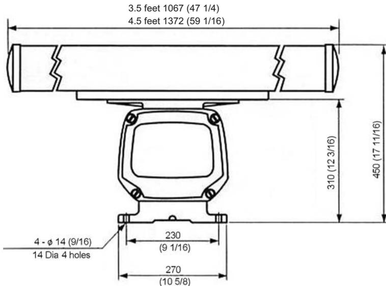
Fig. 4.4 - Radar SWR 10 (1)
