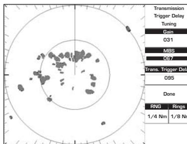
Fig. 1.7.4.4f - Transmission Trigger Delay tuning (VII)
