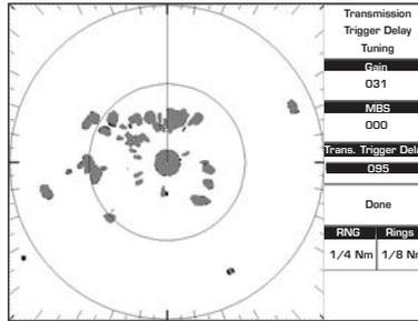
Fig. 1.7.4.4d - Transmission Trigger Delay tuning (V)
