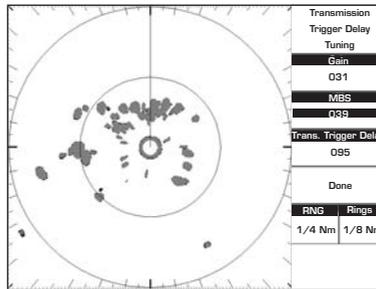
Fig. 1.7.4.4e - Transmission Trigger Delay tuning (VI)
