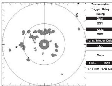
Fig. 1.7.4.4c - Transmission Trigger Delay tuning (IV)
