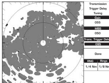
Fig. 1.7.4.4 - Transmission Trigger Delay tuning (1)
