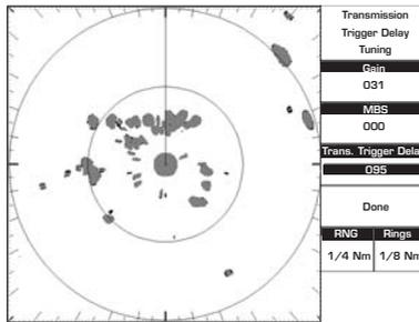
Fig. 1.7.4.4b - Transmission Trigger Delay tuning (III)
