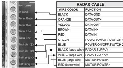
Fig. 1.6a1 - Terminal Strip A Connection for SWR 10
