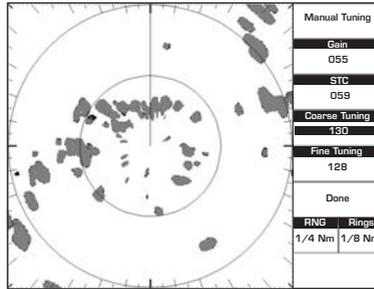
Fig. 1.7.4.5b - Manual Tuning procedure (I)
