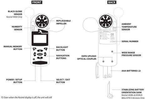
Even when the Kestrel display is off, the unit will still automatically collect and store data at the defined rate (see "Memory Options"). To completely power down the unit, you must remove the batteries (and lose time / date and other settings)
