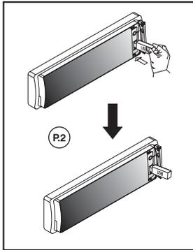
2. Plug in the USB drive / device completely as indicated in picture 2(P.2) and display will show "USB PLAY" to indicate that the USB drive / device is being plugged in correctly & the download has begun.
