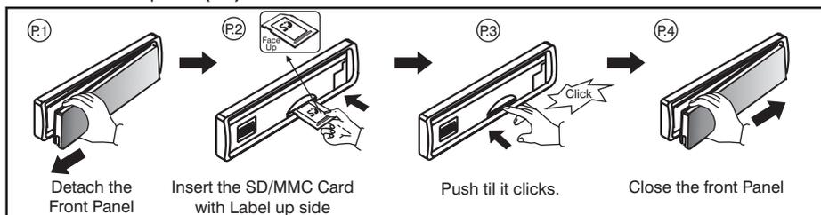
5. The display will show "SD PLAY" to indicate that the SD or MMC card is correctly inserted. Once the SD or MMC card is inserted, the MP3 file will automatically play.
