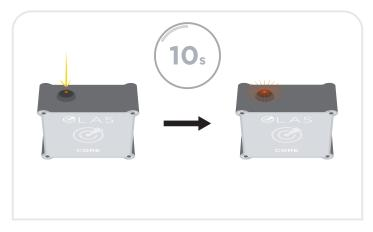
**9.** Press the control switch once. Wait 10 seconds and the system will be operating again. Solid red on the control switch indicates it is tracking correctly.
