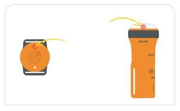
**3.** Switch off the OLAS transmitters. **OLAS tag:** press the button for 4 seconds, until a red flash is seen. **OLAS Float-On:** press the button for 4 seconds until the bi-colour turns red.
