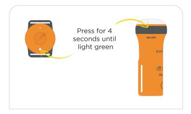
7. Switch the OLAS transmitter back ON.
