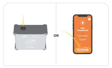
**5.** Press the control switch on the Core once. This puts the system into pause.
