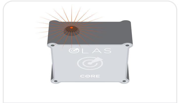
**14.** If no alarm sounds return to the Core and check that the control switch is illuminated red. Solid red indicates that the Core is tracking correctly.
