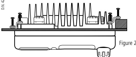
Ensure that the location selected for in dash mounting is convenient for the operator and that there is sufficient space behind the panel to accommodate the body of the radio and allow a free flow of air. Refer to page 13 of the Instruction Manual for more hints.
