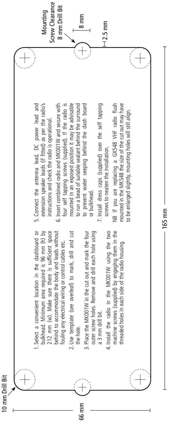
Mark and cut a hole 66 mm (h) by 165 mm (w), allowing for clearance of the two mounting screws holding the radio to the surround.
