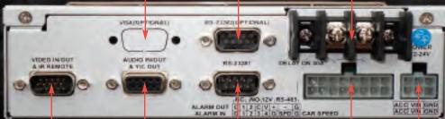
Camera Inputs Monitor Output RC Sensor Audio Inputs / Output Y / C Output
