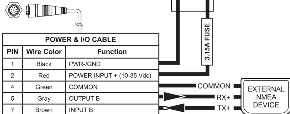
**Note:** NMEA-0183 input baud rate is automatically detected and selected. If you need to set the baud rate manually please go into the settings menu.
