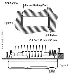
Ensure that the location selected for in dash mounting is convenient for the operator and that there is sufficient space behind the panel to accommodate the body of the radio and allow a free flow of air. Refer to page 13 of the Instruction Manual for more hints.
