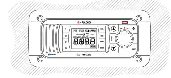
Flush Mounting using the optional MK008 mounting kit.
