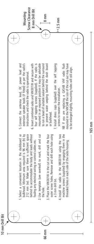
Mark and cut a hole 66 mm (h) by 165 mm (w), allowing for clearance of the two mounting screws holding the radio to the surround. Use a 10 mm drill bit to form the radius of the corners and an 8 mm drill bit for the clearance of the mounting screws.
