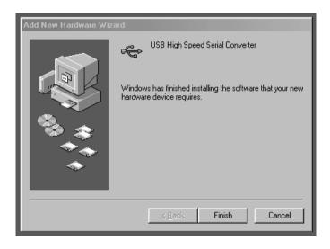
After the USB driver has been installed, it must be optimized using the Windows "Device Manager" before you can use the new driver. To get into the Windows Device Manager:
