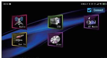
Connect your smartphone to this receiver through Bluetooth, then tap the APP and turn on it on user's smartphone. Now user can control the audio of receiver by the smartphone or tablet.
