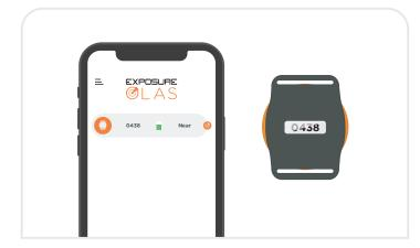
**11.** Check that the tag displayed on the app screen has the same ID number as the tag you are testing with. The tags ID number can be found on the underside of the tag.
