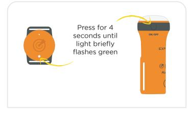
**3.** Switch on 1 x OLAS Tag (or switch on OLAS within the OLAS Float-On).
