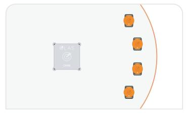
**15.** If you have other OLAS transmitters to track these can now be added to the system. Ensure all OLAS transmitters are switched on and transmitting and place them all within 1 metre of the Core.
