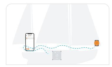
**13.** Walk around your vessel with the tag, listening out for the alarm to sound from the Core or the mobile device.
