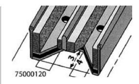
Drain shown above may be made with a saw cut across the bottom and tin snips cuts made parallel to sides. Cut nylon strips to match opening and push into place. Drill 1/8" holes through nylon felt and stainless channel for No. 5 flathead brass screws, 3/4" long. Use 1/16" diameter drill for wood screw pilot holes in framework at 12" centers; screws to be set deep enough into nylon to ensure glass clearance.
