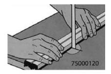
When using band saw on 75000118, 75000119, 75000120 or 75000081, be sure it has a metal cutting blade. Feed into saw slowly with both beads down on work surface.
