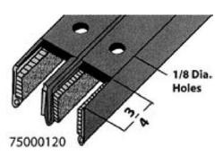
When installing 75000081 edge channel, place rubber glass setting tape (Sealstrip Part# 75000662) over edge of glass. Properly position edge channel over tape and hammer onto glass. To avoid denting channel, place hardwood block against channel and hammer on wood.
