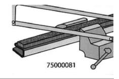
All channels can be cut with hacksaw, except 75000118 (use bandsaw or tin snips). When using a hack saw on 75000119, 75000120, or 75000081, hold the channel in a vise and saw as shown to prevent loosening of pile and beading.
