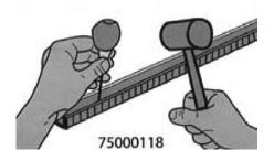
An ice pick or scriber can be used to punch screw holes in the bottom of 75000118. It is recommended that 3/4" x #5 flat-head brass screws on 12" centers be used. Channel should be screwed down deep enough into nylon bottom to assure glass clearance.
