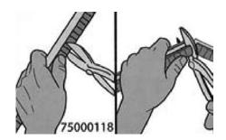
Tin snips can be used to cut 75000118. When using tin snips, cut each side separately, cutting from the bead to the bottom, then fold back the bottom and cut square.
