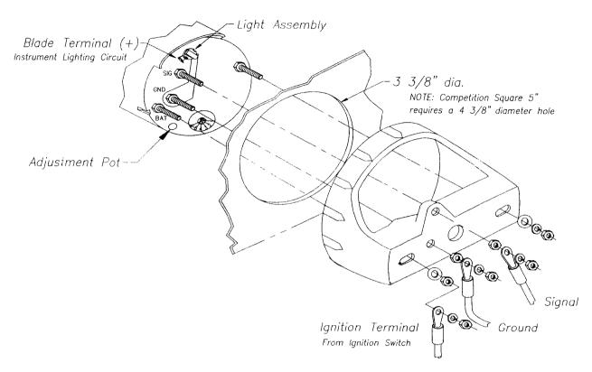
CAUTION: Disconnect the battery during installation. Tighten nuts on the backclamp only slightly more than you can tighten with your fingers. Six inch-pounds of torque is sufficient. Overtightening may result in damage to the instrument and may void your warranty.
